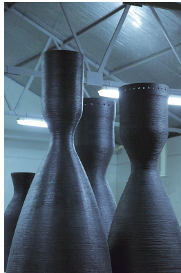
Figure 2.18: Venator (left) and Executor (right) rocket engines nozzles and chambers.
