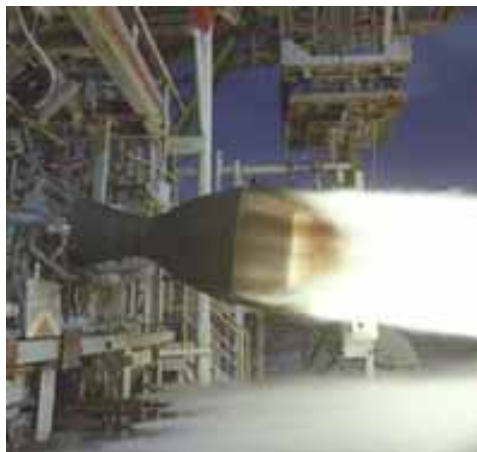
Figure 2.13: Fastrac engine hot-fire test at Marshall Center (NASA/MSFC)
