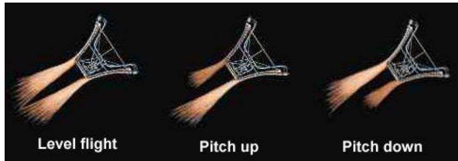
Figure 2.37: TVS (Thrust Vector Control) in Linear Aerospike Engines.
