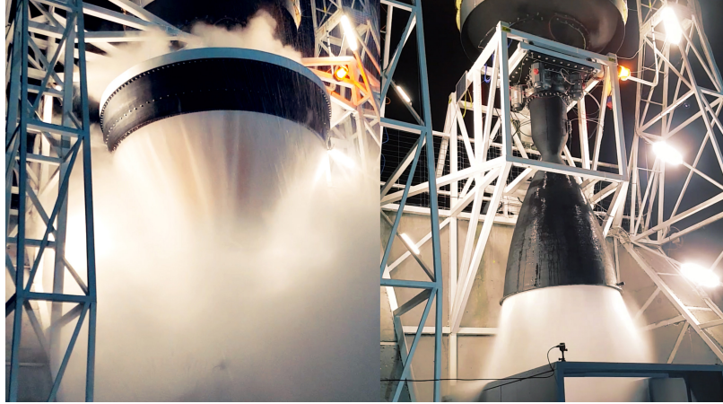
Figure 2.16: Aerospike engine & the classic bell-shape nozzle engine during tests.
